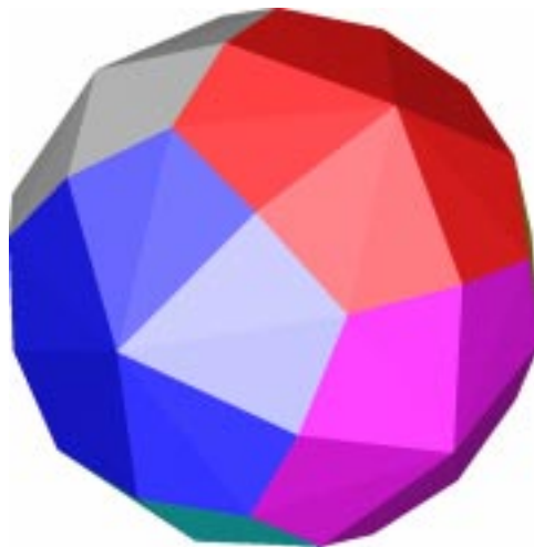
Figure 5.2: The 120-faceted ball \mathcal{B} . Adjacent “plates” of 10 facets have been given different colors for contrast. There are 12 such plates, each centered at one of the vertices of an icosahedron.
